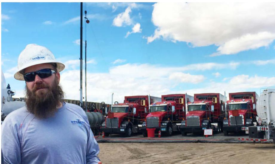
Figure 3. “Quiet fleet” (diesel engines with sound suppression) for hydraulic fracturing. Photo by Jill Engel-Cox, NREL
