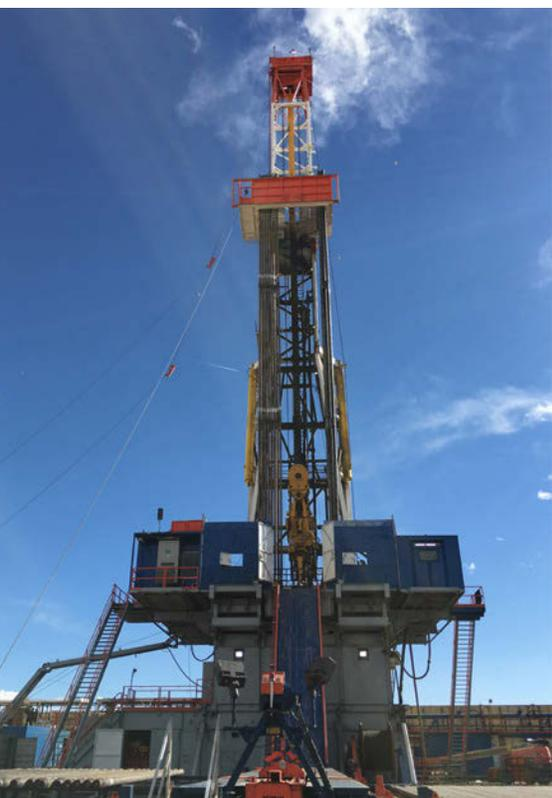
Figure 1. Electric drill rig.
